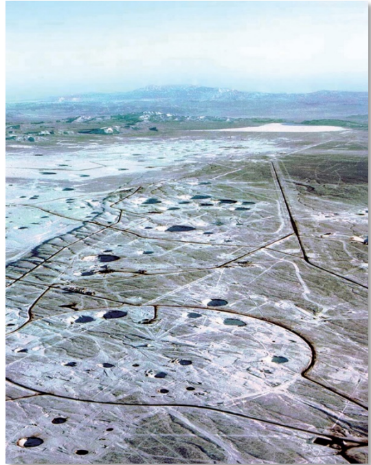
Figure 13.15 Subsidence Craters at Yucca Flats, Nevada National Security Site
